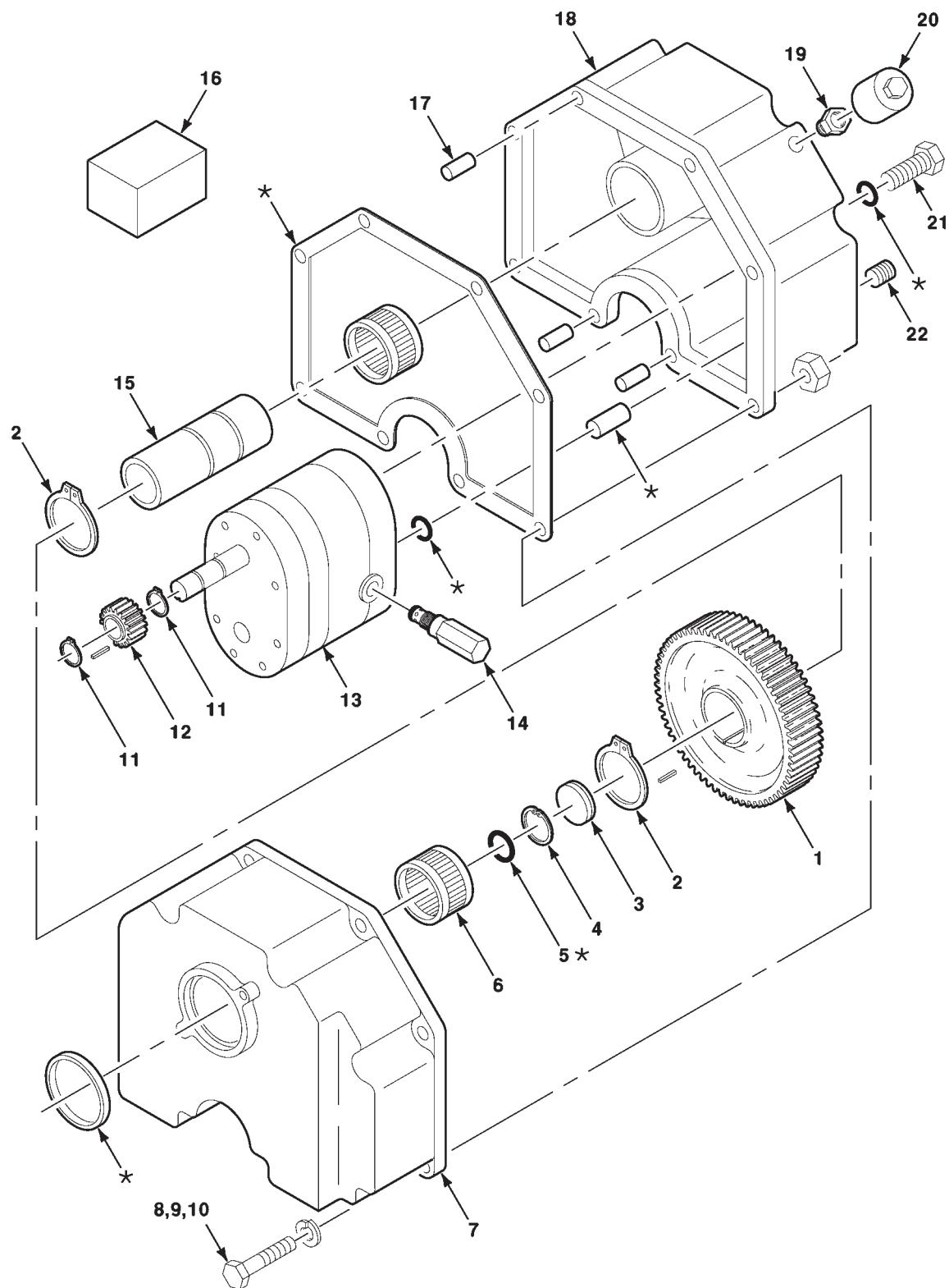
**PTO PUMP ASSEMBLY (540 RPM)**
