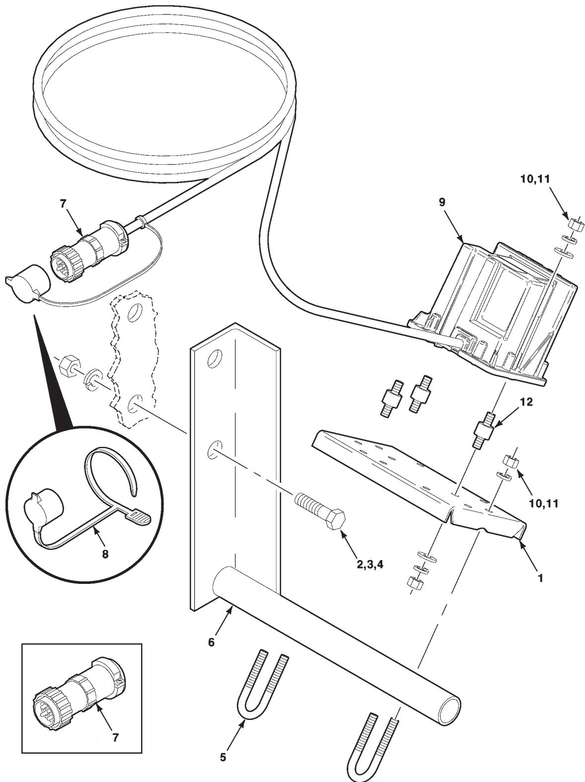
RADAR DISTANCE SENSOR AND MOUNTING
