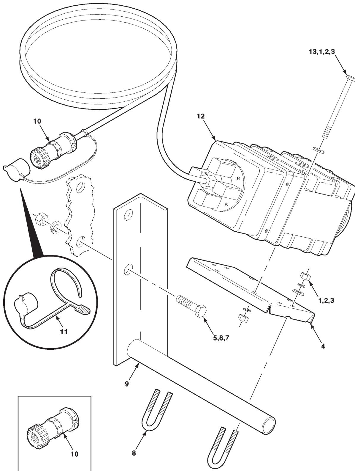
RADAR DISTANCE SENSOR AND MOUNTING
