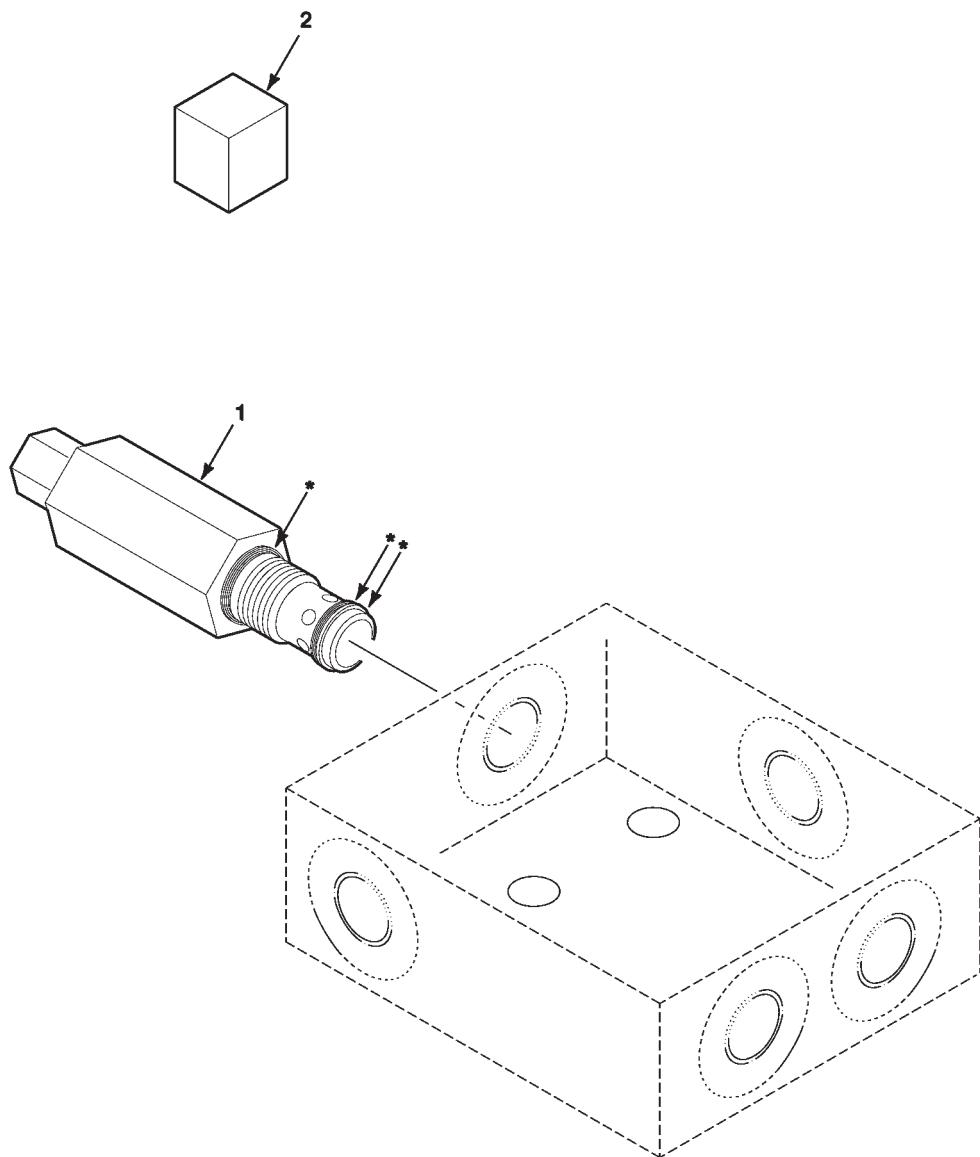
**RELIEF VALVE ASSEMBLY-LIFT ASSIST**
